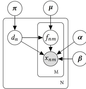
Fig 3. The plate representation of FIRD in discrete space. The parameter  $\pi$  is the mixture weight.  $\mu$  balances the adversarial distribution pairs. The synchronization and randomness are captured by the adversarial distribution pairs, whose parameters are  $\alpha$  and  $\beta$ , respectively.
