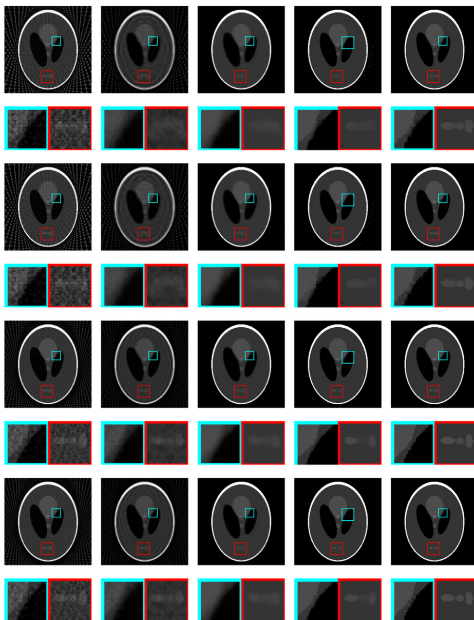
Figure 5. Performance on ‘Shepp–Logan’ images restoration. From top to bottom: 30 projections, 30 projections + noise, 45 projections and 45 projections + noise. From left to right: results of FBP, \ell_2 norm, \ell_e norm [17], \ell_0 norm [1], and ours, respectively.
