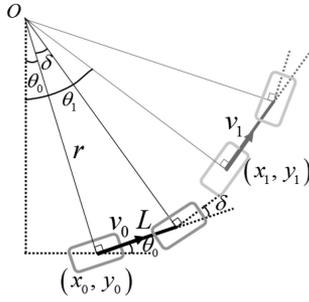
Fig. 2. The vehicle bicycle kinematic model.
